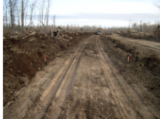
Figure 3: Mobility section rutting after two high tire pressure passes
